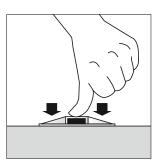
3. Press down firmly on the base with the thumbs for several seconds.
